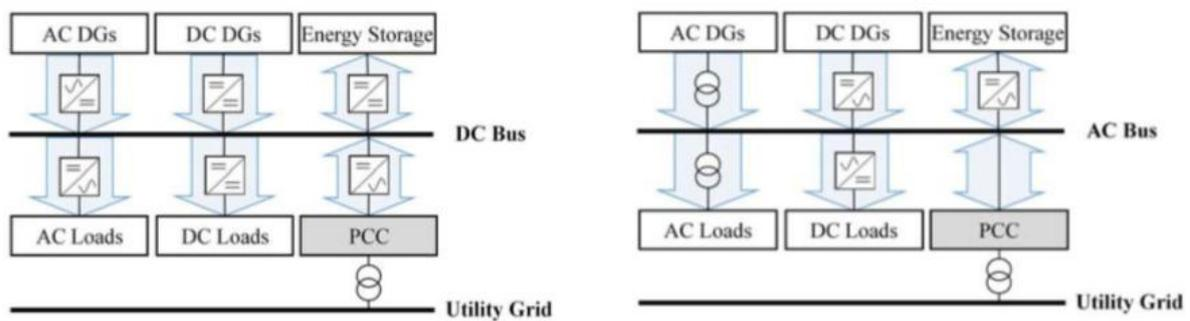
Fig. 1.a) General structure of dc microgrids
