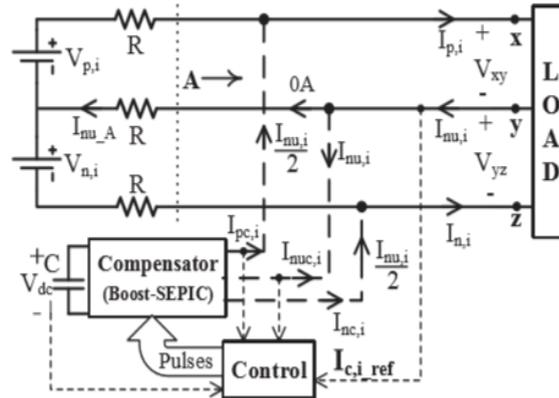
Fig. 3. Circuit with a Boost Sepic converter
